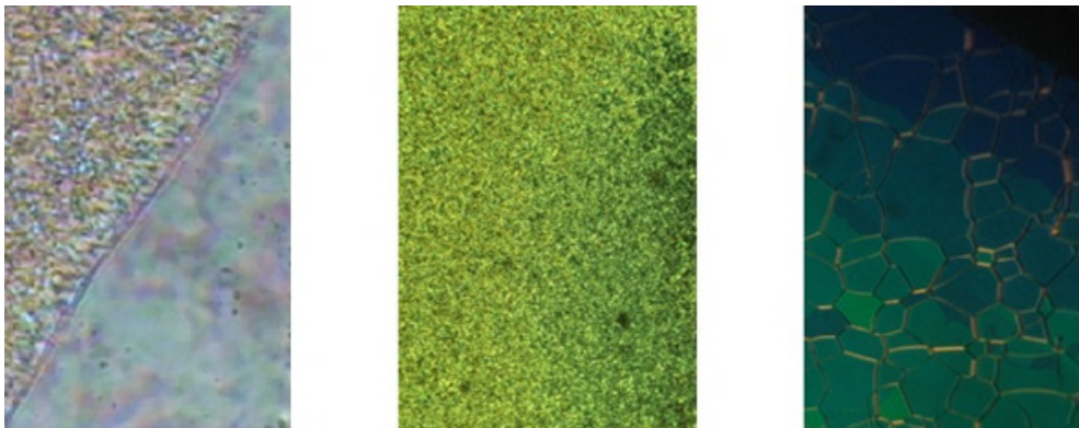
Fig. 18. Left to right: phase transition between the cholesteric phase (left-hand side, top corner) and the blue phase (right-hand side side); the texture of the cholesteric phase; the texture of the cholesteric phase with the texture of the blue phase BP II and BP III [6]
