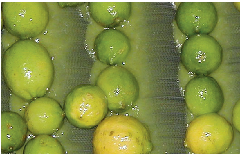
Fig. 41. Rollers of the essential oil extractor with the fruits rotating on them, covered with a thin layer of water [66]
