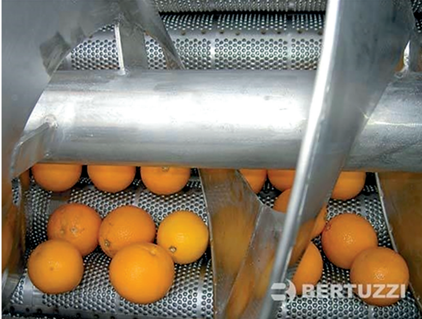
Fig. 32. Interior of a Bertuzzi Citro Rap machine from Bertuzzi, for the Pelatrice process [58]
