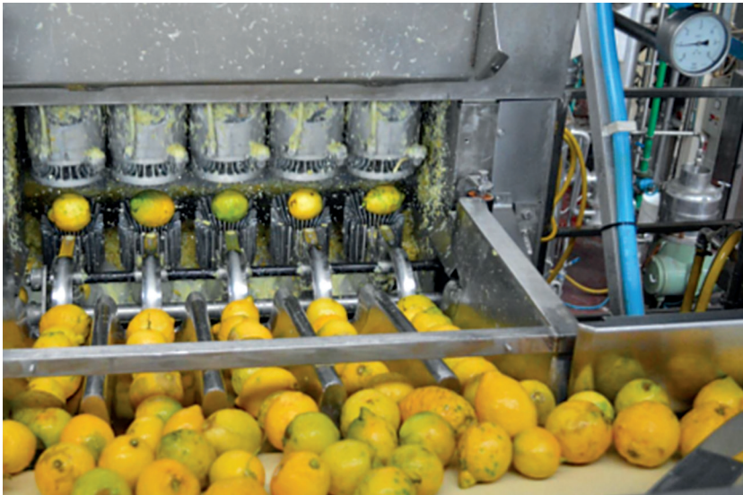
Fig. 38. Photograph of a machine for simultaneous extraction of juice and oil by the FMC method [66]
