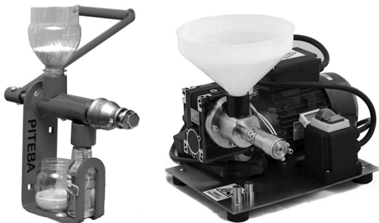
Figure 2.6.2. Two types of laboratory-scale oil extruders – from the left: Piteba hand-press, mechanical PS-10 extruder
