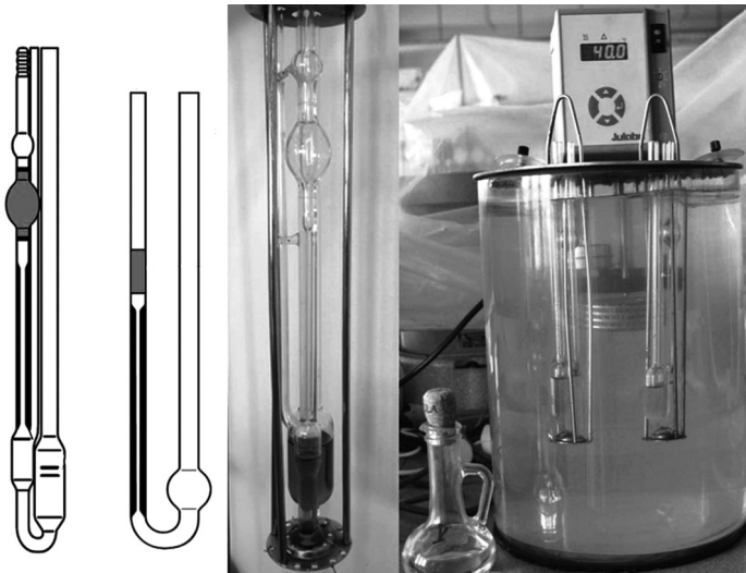
Figure 3.2.3.1. From the left: Ubbelohde and Ostwald capillaries, Ubbelohde capillary in a protective basket, and sample placed in a thermostated water bath. Blue marks the measurement bubble, where the time of liquid flow is measured
