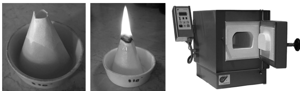
Figure 3.2.9.7. Crucible with liquid sample for ash determination, and muffle furnace for calcination
